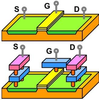
Fig. 1. Diagrams for device-level FET device with complete deembedding (top) and proposed circuit-level FET device with wiring parasitics (bottom).
