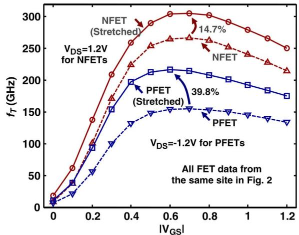
Fig. 3. Stretched and minimum gate-pitch FET  $f_T$  responses with gate voltage  $|V_{GS}|$  sweep from 0 to 1.2 V with 0.1-V step at  $|V_{DS}| = 1.2$  V. The gate-pitch stretching improves NFET  $f_T$  by 14.7% and PFET by 39.8% in this site. Stretched PFET  $f_T$  response shifts slightly to higher  $V_{GS}$  (to left), and the maximum  $f_T$  is sampled at  $V_{GS} = -0.6$  V, whereas NFET maximum  $f_T$ 's are sampled at  $V_{GS} = 0.7$  V.
