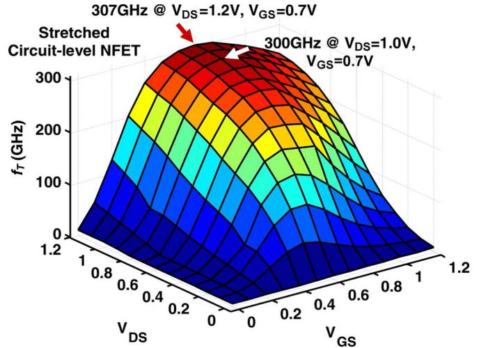
Fig. 2. Circuit-level stretched gate-pitch NFET current gain cutoff frequency  $f_T$  responses with gate voltage  $V_{GS}$  and drain voltage  $V_{DS}$  sweep from 0 to 1.2 V with 0.1-V steps. Maximum of 307 GHz is observed at  $V_{GS} = 0.7$  V and  $V_{DS} = 1.2$  V.  $f_T$  is almost saturated after  $V_{DS} = 1.0$  V, as marked in 300 GHz at  $V_{GS} = 0.7$  V and  $V_{DS} = 1.0$  V. The data were collected at the highest  $f_T$  performance site out of full-wafer measurements.
