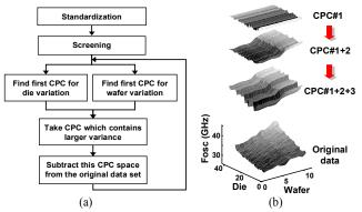
Figure 6. (a) The diagram of the proposed CPCA algorithm. (b) Original data (oscillation frequency of a ring oscillator with respect to die and wafer index for a 65nm technology node and 300mm wafer), CPC#1, CPC#1+#2 and CPC#1+#2+#3.
