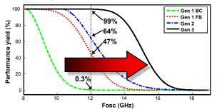
Figure 14. Fosc yield curves for three 65nm technology generations. Each curve represents estimated performance yield with respect to minimum Fosc target. The resulting yields with 12GHz target are shown for each generation. Both BC- and FB-device-based yields are shown for the first generation.
