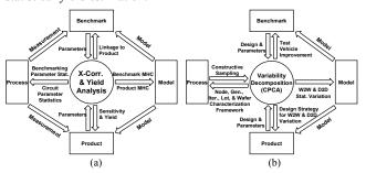
Figure 4. (a) Diagram of parametric statistical analysis (PSA), with enabling development component interactions (b) Diagram of variability decomposition using constrained principal component analysis (CPCA) and its enabling development activities.
