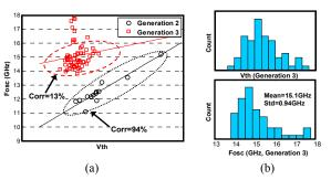
Figure 11. (a) Fosc vs Vth for generations 2 and 3, and their cross-correlations. Each line denotes a linear regression that fits sample points. (b) Histograms of Vth and Fosc in generation 3.
