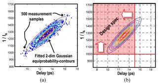
Figure 5. (a) 500 measurement points of reciprocal of active current  $(1/I_A)$  vs delay for a 101-stage RO in 90nm technology and the bi-variate normal distribution fit. (b) Illustration of the yield calculation using integration of volume under a set of design specifications (maximum active current=1mA and maximum delay=15ps).
