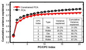
Figure 7. A Cumulative variance of PCA and CPCA for a typical in-line data (1109 parameters for 520 samples – 40 chips for 13 wafers). It shows the cumulative variance which can be explained by first 20 PC's and CPC's using the ordinary PCA and CPCA, respectively. The variation type (die-to-die or wafer-to-wafer) and variance corresponding to the first five CPC's are listed in the table.
