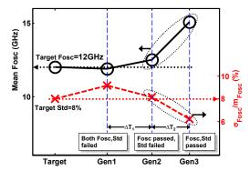
Figure 15. Mean Fosc and standard deviation normalized by mean, over three generations.
