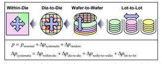
Figure 3. Definition of four ranges of process-induced variability. The systematic variation includes within-die, die-to-die, wafer-to-wafer, and lot-to-lot components.
