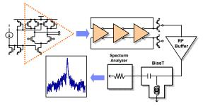
Figure 9. Diagram of a CML inverter in ICO, and measurement set-up for oscillation frequency (Fosc) acquisition.
